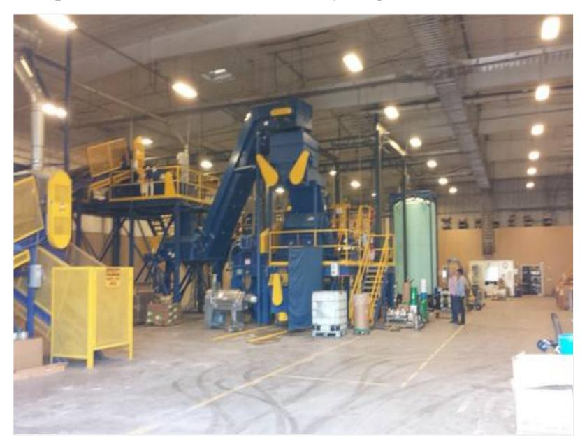
Complete Biomass/Green Waste/Recycling/Tire Shredding Processing Plant with capabilities of running at 20,000 pounds per hour capacity.
